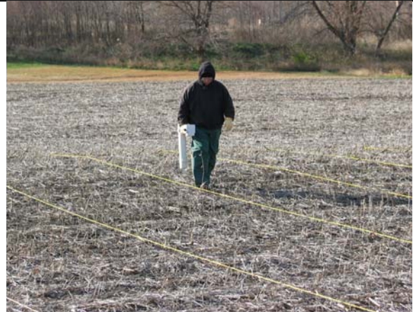
Conducting magnetic survey with fluxgate gradiometer
